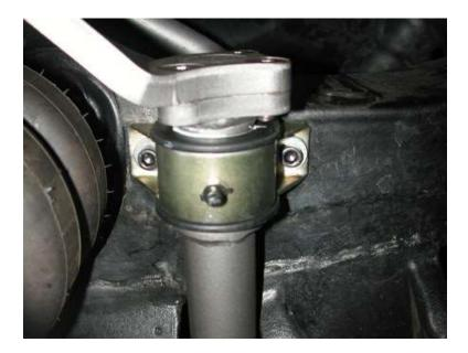
5. Secure the sway bar to the frame with two 5/16" x 1" Socket Head Cap Screws, flat washers and Nylok nuts.
