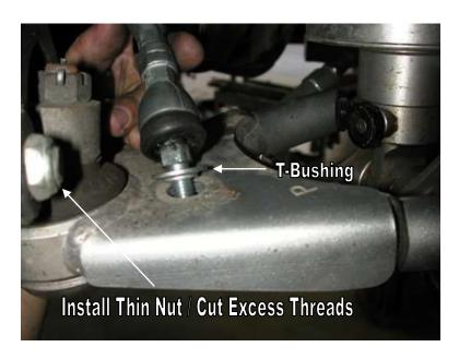
8. The straight end of the PosiLink will attach to the lower control arm.
