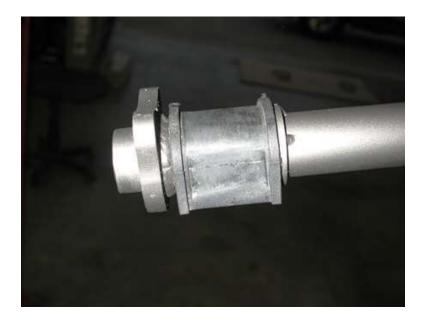
4. Apply lithium grease to the poly bushing then slide it over the sway bar.
