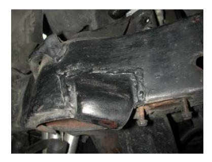
3. On some cars, the compression stop bracket that is welded to the frame will need to be removed to allow clearance for the sway bar arm.
