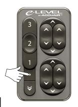
Your system was shipped with the *Tank Pressure Mode* set at **150 PSI**. If you have High Pressure Compressor(s) you can change the *Tank Pressure Mode* to **175 PSI** or **200 PSI** using the following Procedure:
