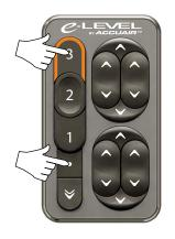
With the Ignition ON, use the Manual Rocker Switches to *Raise/Lower* all four corners until each corner is at your preferred **MAXIMUM TRAVEL** and the vehicle is level from side to side.
