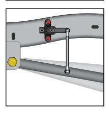
**Step 10.)** Use the final sensor location to mark the two mounting holes to be drilled through the frame. Drill the holes and install the sensor mounting hardware. (**BE CAREFUL NOT OVER TIGHTEN!**)
