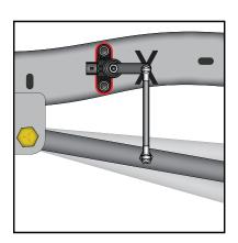
**Step 7.)** Attach the lower end-link to the ball stud. With the vehicle about half way through the travel, find the exact sensor mounting point that keeps the mounting holes and linkage rod vertical. Once established, trace the outline of the sensor to the frame.
