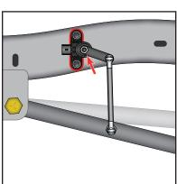
**Step 9.)** With the vehicle at the very top of the travel, compare the clearance found in step 8, to the clearance between the lower plastic stop and the rotating arm. Repeat Step 8 and 9 until the upper and lower clearance is approximately equal.
