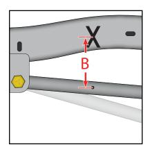
**Step 3.)** While standing clear, exhaust the vehicle to the very bottom of its travel. Now re-measure from your dot up to the center of your "X". We will call this distance "B".
