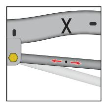
**Step 4.)** If your sensor travel is less than 2.75" then move further away from the pivot point of your suspension arm and repeat steps 1 through 3. If your sensor travel is more than 2.75" then move closer toward the pivot point of your suspension arm and repeat steps 1 through 3.
