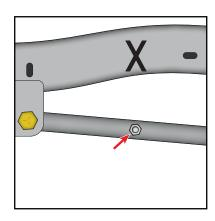
**Step 5.)** Once you have established your ball stud mounting point that yields 2.75" of sensor travel drill or weld to attach the supplied ball stud at this exact point.
