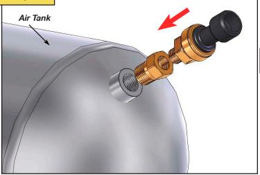
MARNING: e-Level™ System is NOT compatible with any other Pressure Sensor or Switch.
